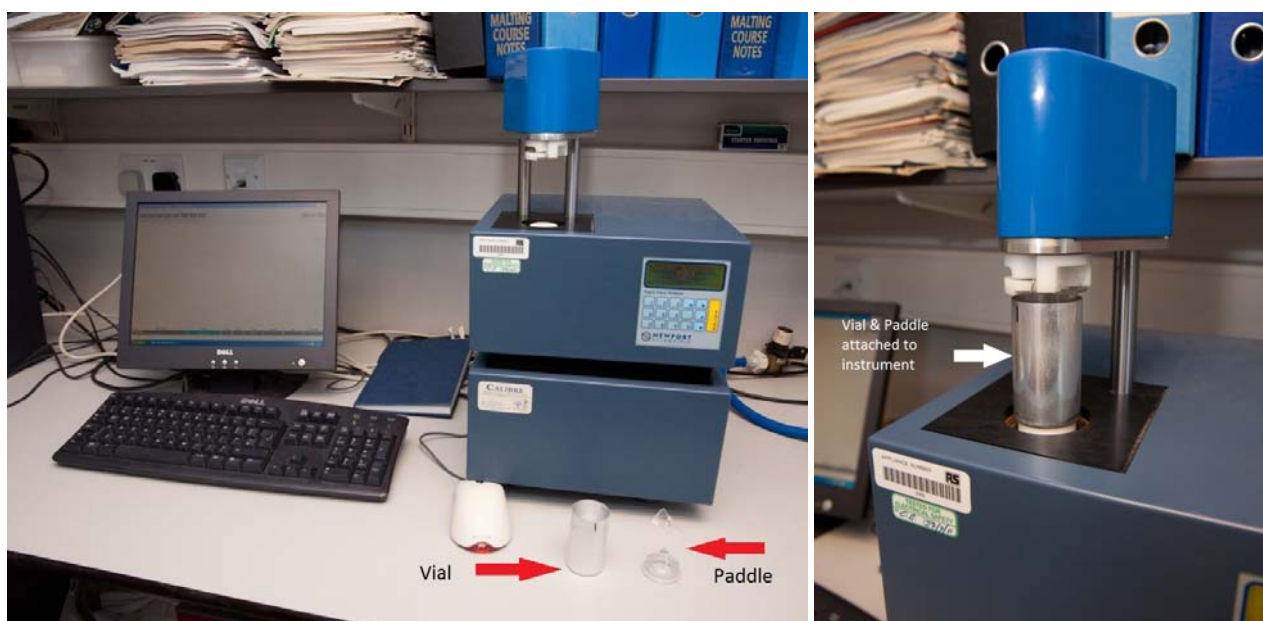
Figure 29. RVA with aluminum vial and plastic paddle on bench (left) and attached to the instrument (right).
