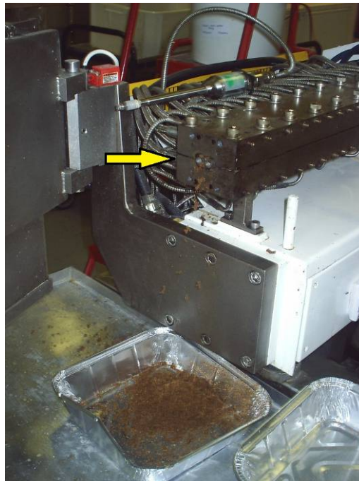
Figure 44. DDGS being extruded through the twin screws and collected in a foil tray.
